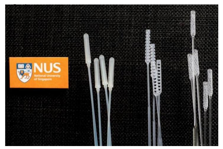
The three nasopharyngeal swab designs can be made using 3D-printing and a manufacturing process known as injection moulding. PHOTO: NATIONAL UNIVERSITY OF SINGAPORE
